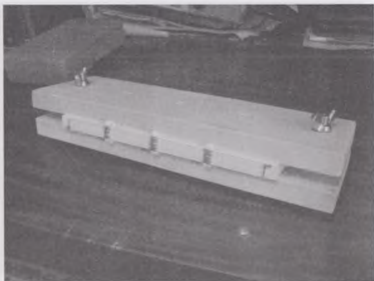
80-rasm. Kitob blokini press yordamida siqib yon tomonini yelimlash
